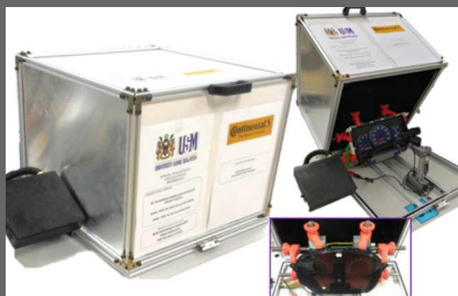
VICTORi - Vehicle Instrument Cluster Test Operation in Real-time Inspection
